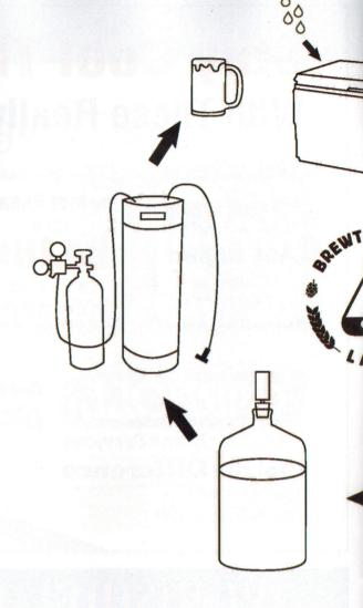
This is a diagram of the brewing process, with the Brewtherville Labs' logo in the center. Brewing starts by adding hot water and grain to a cooler, then transfering that to another tank and adding yeast, putting it through two fermentation processes and finishing it up in a keg. Photo courtesy of Brewtherville Labs
